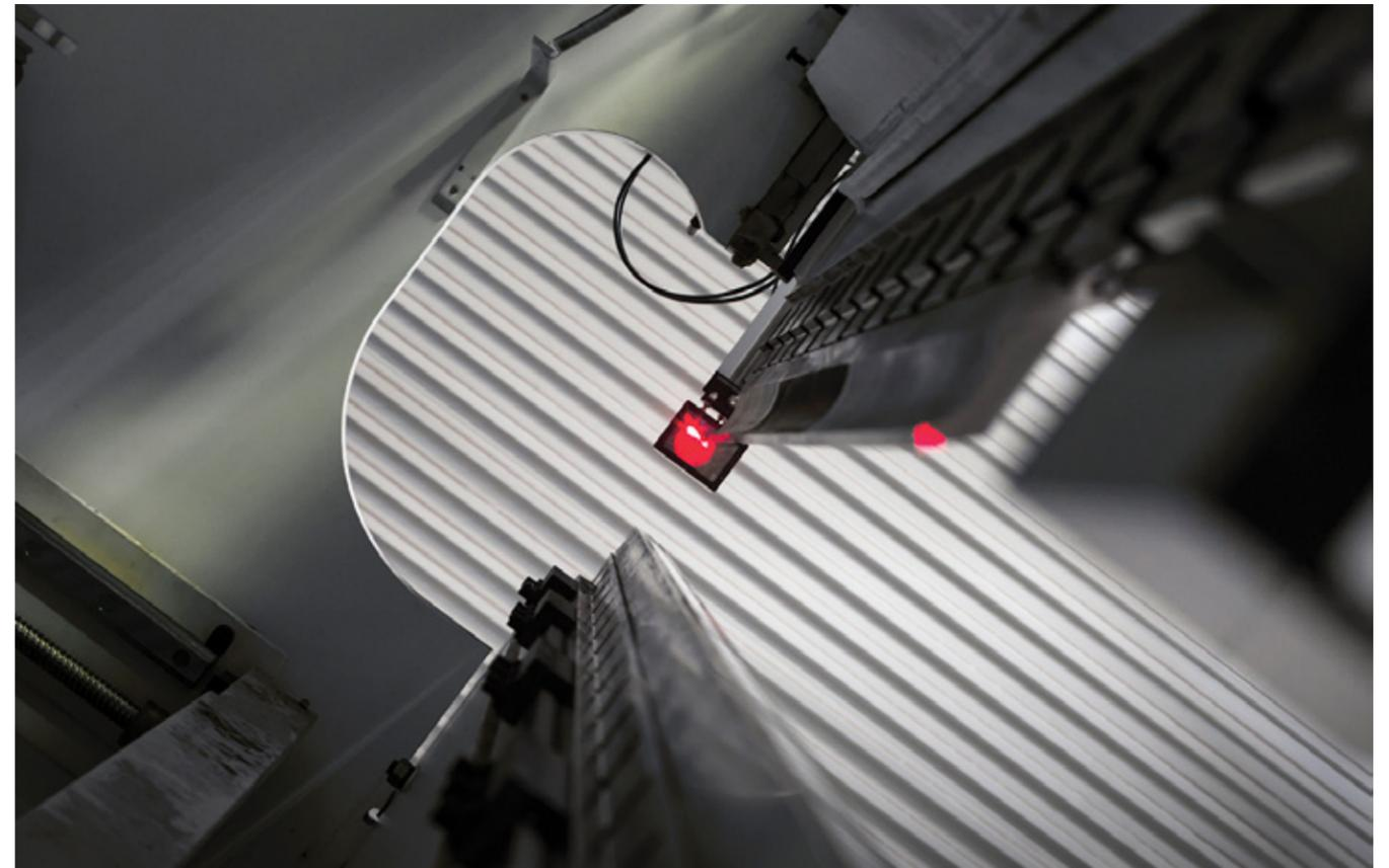
flattening tools with different profiles will result in different protective configurations.
