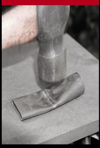
(although it's less abrupt than with MIG). It will crack, they say. The fact is, TIG is used in the large majority of ground vehicle and air frames, with no problems. Myth No. 4: You have to "stress relieve" welded joints with an oxyfuel torch or rosebud. As the article explains, that's only true in thicker sections. Most welding of 4130 is performed on thin-walled tubes, and they don't require stress relieving.
