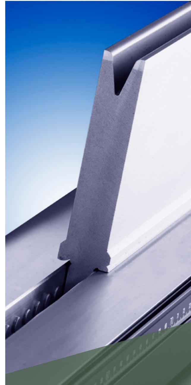
Shown here is a 3.937-in.- (100-mm) tall acute angle die with a large radius on the shoulders to reduce die marking.
