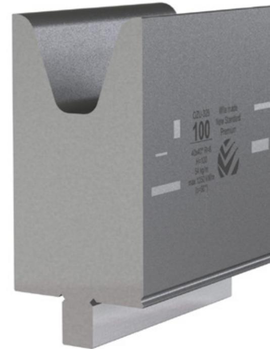
← Shown here is an acute angle single V die with a 1.575-in. (40-mm) V-opening. Note the large 0.315-in. (8.0-mm) radius on the shoulders to reduce die marking.
