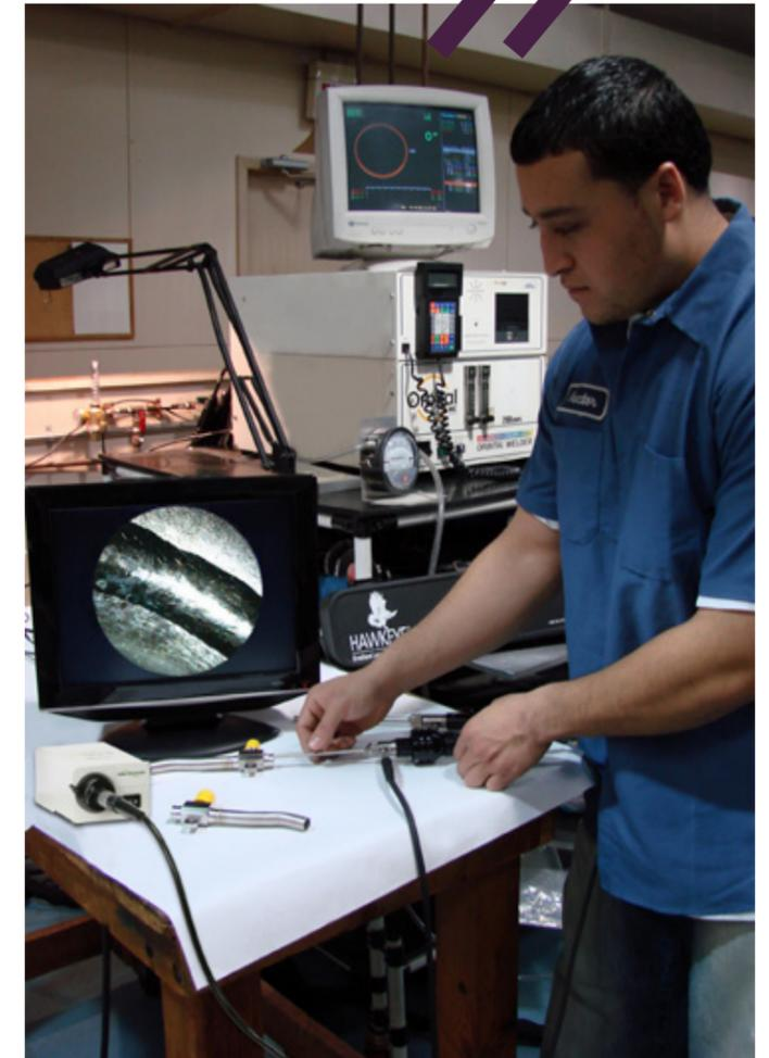
*Aircraft parts manufacturer Kreisler Mfg. checks the welds of parts as early in the process as it can.*
