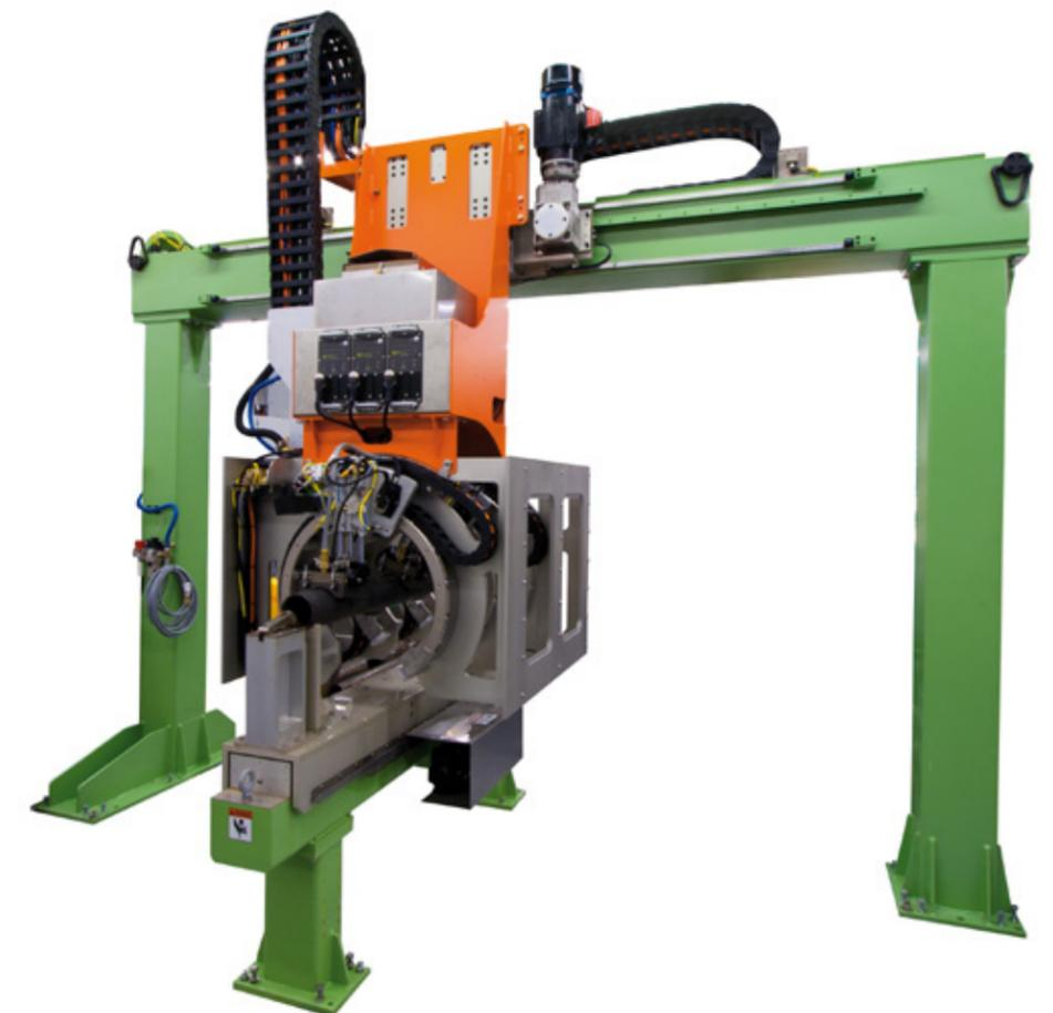
inline or offline when performing inspections, automatic calibrations or maintenance operations. The head rotation capability allows each probe independent movement from -120 to +120 degrees for weld tracking.
